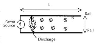
The parameters of the system are the following: length L=1 m, distance between the rails  $\ell=0.1$  m, current i=10 A, field B=1 T. The plasma discharge consists of  $10^{13}$  Hydrogen ions, the mass of a single ion is  $m_H=1.6710^{-27}$  kg.
