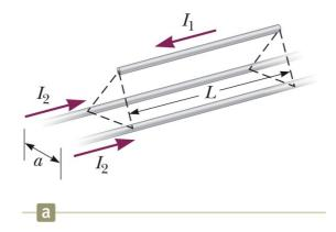
Two infinitely long, parallel wires are lying on the ground a distance a = 12.5 cm apart. A third wire, of length L = 100.0 m, and mass 35.0 kg, carries a current of  $I_t = 1000$  A, and is levitated above the first two wires at a horizontal position midway between them, as can be seen in the figure. The two parallel wires carry equal currents ( $I_2$ ) in the opposite direction to that flowing through the levitated wire.
