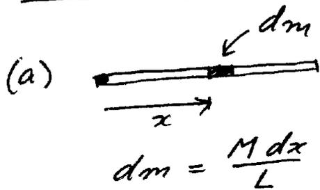
$$\begin{aligned} I &= \int r^2 dm \\ &= \int_0^L x^2 \frac{M dx}{L} \\ &= \frac{M}{L} \left[ \frac{1}{3} x^3 \right]_0^L = \frac{1}{3} ML^2 \end{aligned}$$
