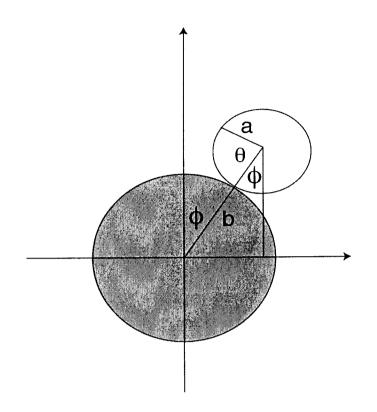
A sphere of radius *a* and mass *m*, with moment of inertia  $I = \frac{2}{5}ma^2$ , rests on top of a fixed sphere of radius *b*. The first sphere is slightly displaced so that it rolls without slipping down the second sphere.
