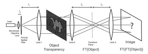
(vi) Using Fourier theory or otherwise, describe the Fraunhofer diffracted field produced by this transparency (camel shape sampled by a 2D array of  $\delta$  functions). This is the field in the back focal plane of Lens 2.
