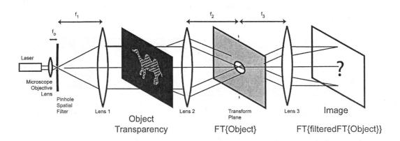
(vii) Using Fourier theory (or otherwise), determine the new image produced by Lens 3 after the diffracted field is filtered by the circular hole mask.
