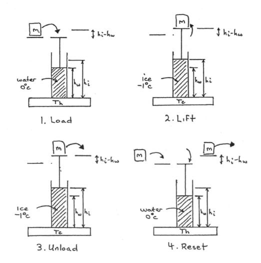
The inventor is pleased with this device because it can seemingly perform an unlimited amount of work (by lifting an unlimited mass m) while absorbing only a finite amount of heat each cycle.
