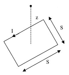
(ii) Derive an expression for the **B** field at a distance Z above the centre of the loop and perpendicular to the loop.
