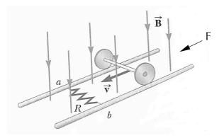
The Figure shows a rolling axle of length 1.50m travelling at a constant speed v=5.00m/s along rails. A 0.200 ohm resistor R is placed between points a and b as shown. You can assume that the rails, wheels and axle are conductors with zero resistance and make good electrical contact with each other. A uniform magnetic field, B, of strength 5.0  $\times 10^{-4}$  T is directed vertically downwards.
