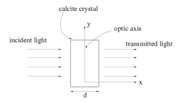
The incident light is linearly polarized with electric field given by the following formula
