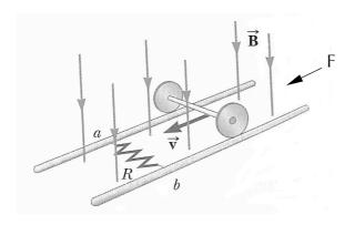
The Figure shows a rolling axle of length 1.50m travelling at a constant speed v=5.00m/s along rails. A 0.200 ohm resistor R is placed between points a and b as shown. You can assume that the rails, wheels and axle are conductors with zero resistance and make good electrical contact with each other. A uniform magnetic field, B, of strength  $5.0 \times 10^{-4}$  T is directed vertically downwards.
