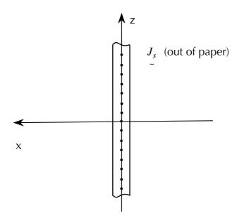
Consider an infinite conducting sheet lying in the yz-plane, as shown in the Figure (the y-axis comes out of the plane of the paper). Suppose the sheet is carrying a uniform current in the y direction, out of the plane of the paper. Let  $J_s$  be the linear current density, i.e., the current per unit length measured along the z axis. The dots in the figure show the current direction (i.e., out of the plane of the paper).
