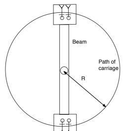
This is a sketch of a circus ride. A beam connects two carriages, in which people ride, secured by seatbelts. The beam rotates about a horizontal axis through its centre, so that the path of the carriages is a circle, radius R, in a vertical plane (as shown). The mass of the carriage (passengers included) is m. The mass of the beam is negligible compared to that of the carriages and the size of the carriages is negligible compared to the length of the beam.
