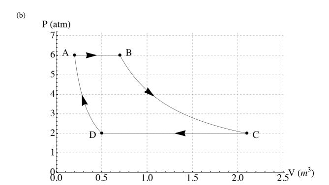
A sample of ideal gas undergoes the process shown in the diagram above. From  $A \to B$  the process is isobaric and 100 kJ of heat enters the system. From  $B \to C$  the process is isothermal. From  $C \to D$  the process is isobaric and 200.0 kJ of heat energy leaves the system. From  $D \to A$  the process is adiabatic.
