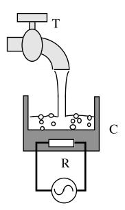
Water at temperature 25°C flows from a tap T into a heated container C. The container has a heating element (a resistor R) which is supplied with electrical power, P, that may be varied.
