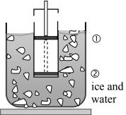
Sketch a Pressure-Volume diagram showing the changes that have taken place, and indicate briefly what thermodynamic processes are taking place at each stage around one complete cycle. If 200g of ice are melted during one cycle, how much work has been done on the gas?
