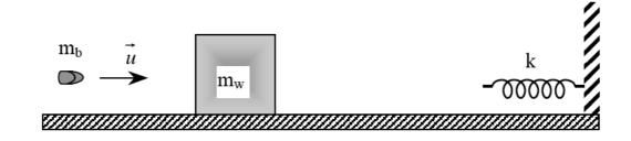
The masses of the bullet and the wooden block are  $m_b = 4.50$ g and  $m_w = 1.63$  kg, respectively.
