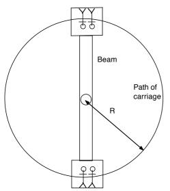
This is a sketch of a circus ride. A beam connects two carriages, in which people ride, secured by seatbelts. The beam rotates about a horizontal axis through its centre, so that the path of the carriages is a circle, radius R, in a vertical plane (as shown). The mass of the carriage (passengers included) is m. The mass of the beam is negligible compared to that of the carriages and the size of the carriages is negligible compared to the length of the beam.
