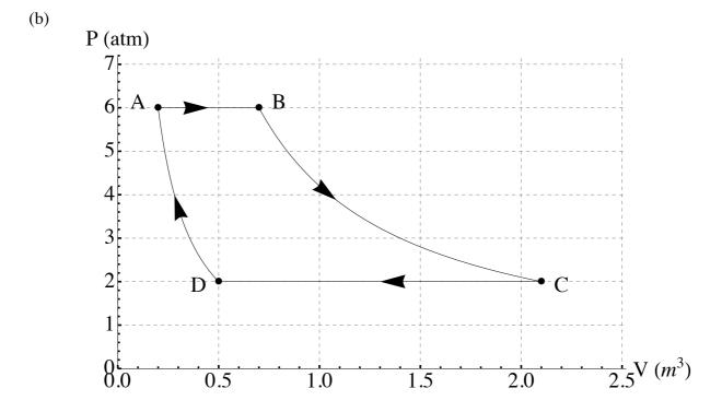
A sample of ideal gas undergoes the process shown in the diagram above. From  $A \rightarrow B$  the process is isobaric and 100 kJ of heat enters the system. From  $B \rightarrow C$  the process is isothermal. From  $C \rightarrow D$  the process is isobaric and 200.0 kJ of heat energy leaves the system. From  $D \rightarrow A$  the process is adiabatic.
