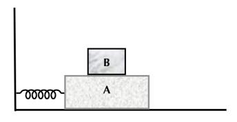
Determine the maximum amplitude of oscillation that block A can have, if there is no relative motion between blocks A & B.
