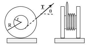
A string is attached to the drum (radius r) of a spool (radius R) as shown in side and end views here. (A spool is device for storing string, thread etc.) A tension T is applied to the string at angle  $\theta$  above the horizontal. The coefficients of kinetic and static friction between floor and spool are  $\mu_k$  and  $\mu_s$  respectively. We are interested in whether and when the spool will move left or right, and how this depends on the nature of the floor.
