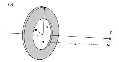
Calculate the electric potential at a point P on the axis of the annulus shown in the figure. The annulus has a surface charge density  $\sigma$ . Its inner radius is a and its outer radius is b. Point P is a distance x away from the centre of the annulus.
