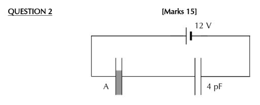
Capacitor A in the diagram consists of square plates with side length 2 cm. separated by 0.5 cm. Capacitor A is filled with a non-conducting liquid, dielectric constant 3.0, to a height of 1.5 cm.
