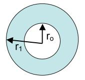
Suppose that  $r_0=5.0$  cm,  $r_1=10$  cm and the coefficient of linear expansion is  $2.0 \times 10^{-5} \text{ °C}^{-1}$ . What is the change in the area of the material that makes up the disk for a 30 °C increase in its temperature?
