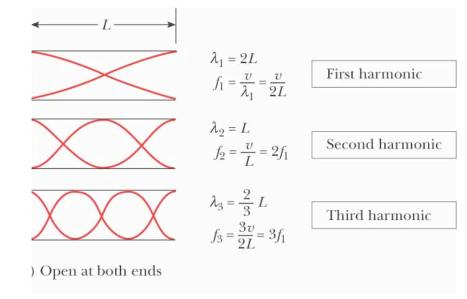
Shown are the first three resonances (or harmonics). Each end of the pipe is an antinode since it is open. We see that  $f_n = nc/2L$  where c is the wavespeed and n=1, 2, 3, ....
