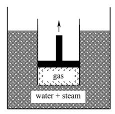
An ideal gas is enclosed by a cylinder with a movable piston. The cylinder is submerged in a mixture of water and steam at 100 °C. The piston is pulled rapidly, increasing the volume of the gas. The piston is held still until the temperature of the gas is again100 °C. Then it is slowly pushed back to the original position. 52.0g of water in the mixture vaporise in the process.
