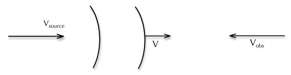
Thus,  $f_{\text{observer}} = f_{\text{source}} \frac{v + v_{\text{Observer}}}{v - v_{\text{source}}}$  from the Doppler formula
