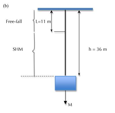
(i) Block is in the free fall when only under the influence of gravity. i.e., for the first 11.0m of the fall, when the cord does not retard its motion
