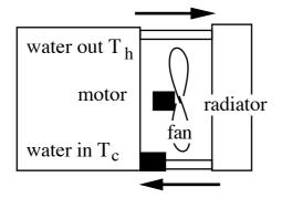
The same car motor has an efficiency of 25%, which we assume to be constant, independent of the speed of the car. So, when it produces 20 kW of power, it produces heat at a rate of 60 kW. We assume that all of this heat is transferred by water in the cooling system to the radiator, where it is transferred to the air passing through the radiator, as indicated in the sketch, where arrows show the direction of water flow.
