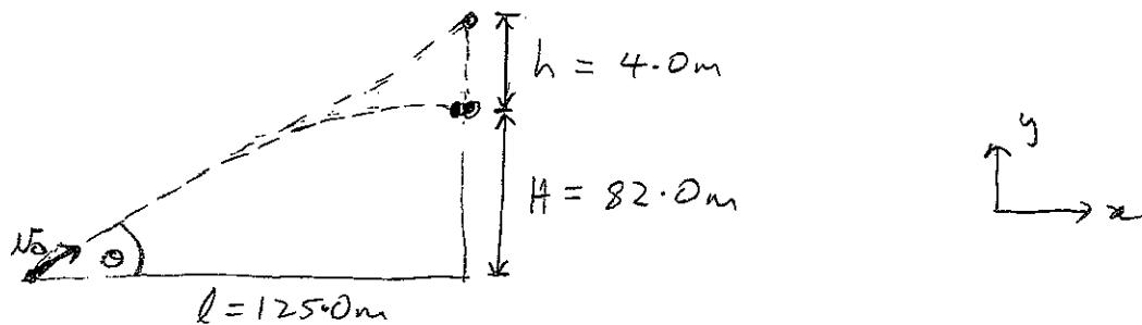
$$(i) \text{ Initial speed of cannon-ball } V_0 = \sqrt{V_{0x}^2 + V_{0y}^2}$$
