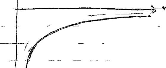
(e) Minimum energy required to separate particles to infinity is energy to give total mechanical energy  $E=0$
