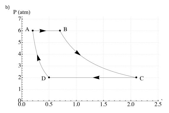
A sample of ideal gas undergoes the process shown in the diagram above. From  $A \rightarrow B$  the process is isobaric and 100 kJ of heat enters the system. From  $B \rightarrow C$  the process is isothermal. From  $C \rightarrow D$  the process is isobaric and 200 kJ of heat energy leaves the system. From  $D \rightarrow A$  the process is adiabatic.
