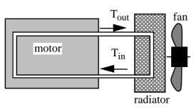
An internal combustion engine (the motor in a car) generates heat at a rate of 20 kW. It is cooled by water that flows in a continuous circuit through a radiator and the motor, as shown in the very simplified sketch. (The radiator dissipates the heat because cool air is forced through the radiator by a fan. This detail is not relevant to our problem.)
