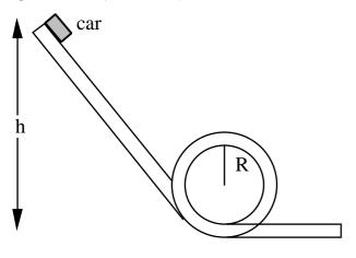
A toy racing car is placed on a track, which has the shape shown in the diagram. It includes a loop, which is approximately circular with radius R. The wheels of the car have negligible mass, and turn without friction on their axle. You may also neglect air resistance. The dimensions of the car are much smaller than R.
