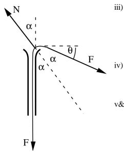
The tension in both ends of the string is F, so, from symmetry, the line of N bisects the angle between the segments of the string. So N is at an angle to the vertical
