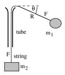
Two masses,  $m_1$  and  $m_2$ , are attached to opposite ends of a string that passes through a tube, whose upper end has been smoothed to reduce the sliding friction with the string. The tube is held vertically and stationary.  $m_1$  is caused to travel in a horizontal circle, in such a way that  $m_2$  does not move. Neglecting the friction between string and tube,
