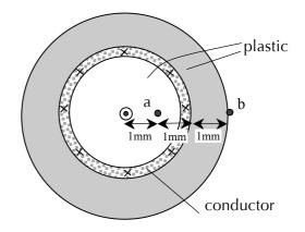
Determine the magnitude and direction of the magnetic field at points *a* and *b*, which are 1 mm and 3 mm, respectively from the centre of the cable, along the positive *x*-axis.
