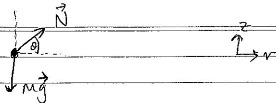
(b). The normal force (projection onto the horizontal) is responsible for the circular motion.
