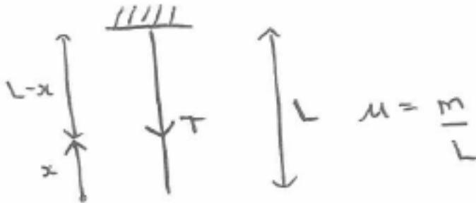
Let the Tension be  $T$  at a distance  $x$  from the end, as in the diagram.
