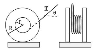
A string is attached to the drum (radius r) of a spool (radius R) as shown in side and end views here. (A spool is device for storing string, thread etc.) A tension T is applied to the string at angle  $\theta$  above the horizontal. The coefficients of kinetic and static friction between floor and spool are  $\mu_k$  and  $\mu_s$  respectively. We are interested in whether and when the spool will move left or right, and how this depends on the nature of the floor.
