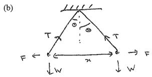
(i) There are three forces acting on each charge, the electrostatic repulsion between the two charges, F, its weight due to gravity, W, and the tension in the silk thread, T.
