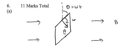
Suppose the axis of the coil makes an angle  $\theta$  with the direction of the magnetic field at time t. Then  $\theta = \omega t$ .
