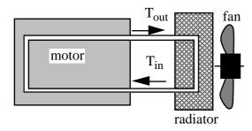
An internal combustion engine (the motor in a car) generates heat at a rate of 20 kW. It is cooled by water that flows in a continuous circuit through a radiator and the motor, as shown in the very simplified sketch. (The radiator dissipates the heat because cool air is forced through the radiator by a fan. This detail is not relevant to our problem.)
