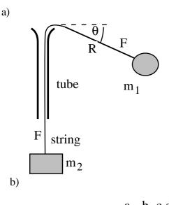
Two masses,  $m_1$  and  $m_2$ , are attached to opposite ends of a string that passes through a tube, whose upper end has been smoothed to reduce the sliding friction with the string. The tube is held vertically and stationary.  $m_1$  is caused to travel in a horizontal circle, in such a way that  $m_2$  does not move. Neglecting the friction between string and tube,
