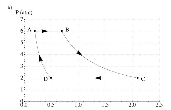
A sample of ideal gas undergoes the process shown in the diagram above. From  $A \to B$  the process is isobaric and 100 kJ of heat enters the system. From  $B \to C$  the process is isothermal. From  $C \to D$  the process is isobaric and 200 kJ of heat energy leaves the system. From  $D \to A$  the process is adiabatic.
