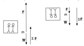
i) Applying Newton's 2nd law to the carriage at the bottom and top:
