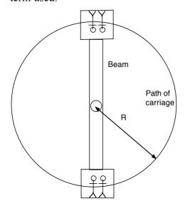
c) This is a sketch of a circus ride. A beam connects two carriages, in which people ride, secured by seatbelts. The beam rotates about a horizontal axis through its centre, so that the path of the carriages is a circle, radius R, in a vertical plane (as shown). The mass of each carriage (passengers included) is m. The mass of the beam is negligible compared to that of the carriages and the size of the carriages is negligible to that of the length of the beam
