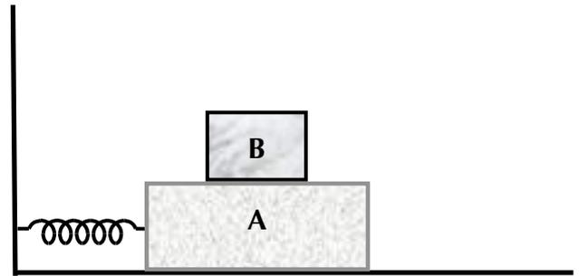
Determine the maximum amplitude of oscillation that block A can have, if there is no relative motion between blocks A & B.
