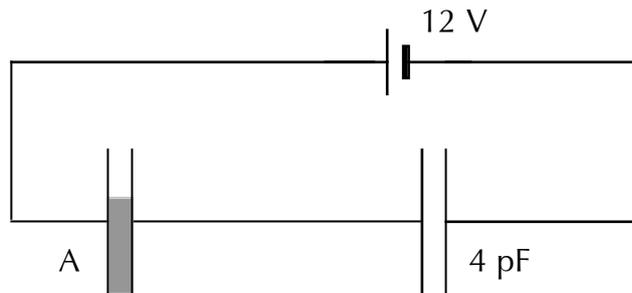
Capacitor A in the diagram consists of square plates with side length 2 cm, separated by 0.5 cm. Capacitor A is filled with a non-conducting liquid, dielectric constant 3.0, to a height of 1.5 cm.
