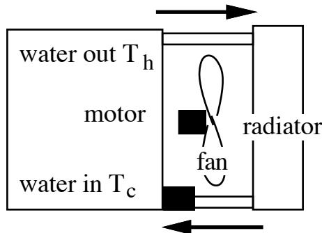
The same car motor has an efficiency of 25%, which we assume to be constant, independent of the speed of the car. So, when it produces 20 kW of power, it produces heat at a rate of 60 kW. We assume that all of this heat is transferred by water in the cooling system to the radiator, where it is transferred to the air passing through the radiator, as indicated in the sketch, where arrows show the direction of water flow.
