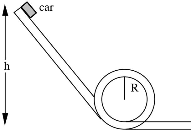
A toy racing car is placed on a track, which has the shape shown in the diagram. It includes a loop, which is approximately circular with radius  $R$ . The wheels of the car have negligible mass, and turn without friction on their axle. You may also neglect air resistance. The dimensions of the car are much smaller than  $R$ .
