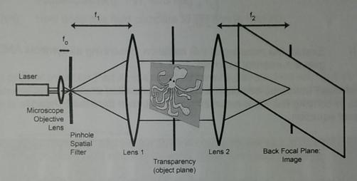
After recording this intensity distribution, the octopus transparency is then rotated 180° about the optical axis. The camera then records the intensity distribution in the back focal plane for the rotated octopus transparency,  $I_{180^{\circ}}(\zeta,\eta)$ .
