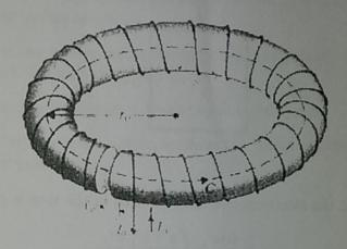
(a) Using the appropriate Maxwell equation, show that the magnetic field inside the ferromagnetic material,  $\vec{B}_f$ , and the magnetic field in the air gap,  $\vec{B}_g$ , satisfy
