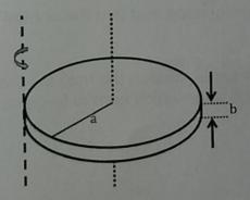
A solid disc of mass, M, radius, a, and thickness, b, rotates about an axis that touches its rim and is parallel to its symmetry axis.
